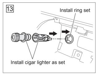
Re-install the removed parts
